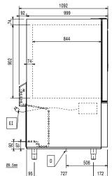
Drain FΙ Electrical inlet (power) Refrigerant Outlet
